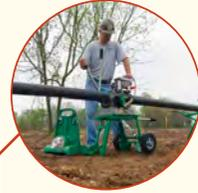
Optional Manual Fusion Machine Stand expands to a comfortable operator level and folds for easy storage when not in use
