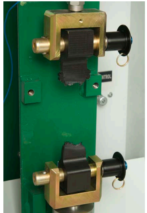
McElroy McSnapper Tested Coupon
