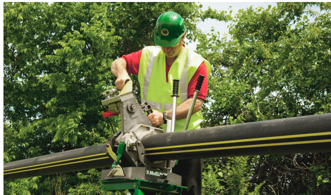
The new McElroy PitBull 26 (left). The PitBull 26 is used with the Manual Fusion Machine Stand and PitBull 26 Productivity Package to bring the fusion machine to a comfortable operating height during fusion operations (top).
