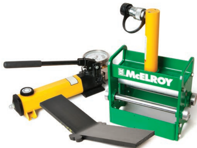
The McElroy Guided Side-Bend Tester sits behind a coupon that passed the quality assurance test.
