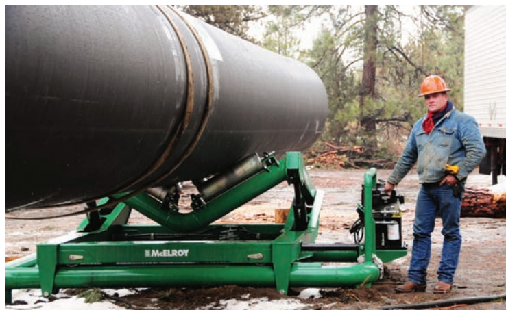
The MegaMc Pipe Stands were recently used on a job in Oregon where workers claimed saving 30 minutes per fusion joint.
