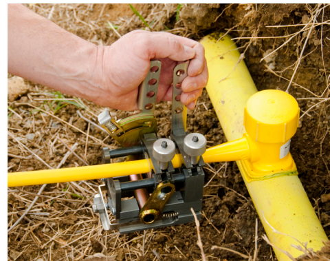
The new McElroy 1LC (left). The 1LC brings two ends of pipe together to complete a butt fusion joint (above).
